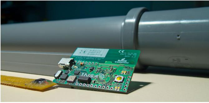
**Figure 2: Components close-up of a snowpack monitoring node: INGA WSN node (middle), temperature probe rod (foreground), enclosure (background)**
